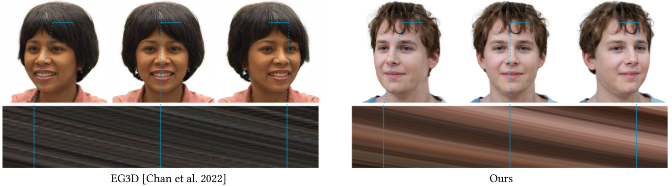
Fig. 6. Analysis of 3D Consistency: We show spatio-temporal line textures akin to the Epipolar Line Images (EPI) [Bolles et al. 1987] obtained by rotating the camera horizontally and stacking the pixels of a fixed horizontal line segment. EG3D suffers from texture-sticking artifacts due to its use of a 2D super-resolution network, leading to staircases in the epipolar line images. In contrast, our method provides smooth renderings without any flickering.
